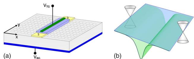
FIG. 1. (Color online) (a) A schematic of a Gedanken experiment for the observation of localized modes in graphene waveguides, created by the top gate ( $V_{TG}$ ). The Fermi level is set using the back gate ( $V_{BG}$ ) to be at the Dirac point ( $\epsilon_F=0$ ). (b) The electrostatic potential created by the applied top-gate voltage. The plane shows the Fermi-level position at  $\epsilon_F=0$ .
